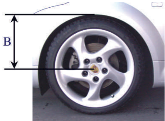
Measurement B Wheel hub center wheel arch
