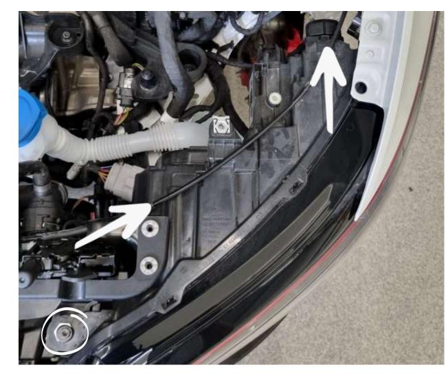
On the cars right side remove 4x T30 screws and remove the hood pin and put it somewhere that will prevent the hood from falling down. Remove the headlight frame.
