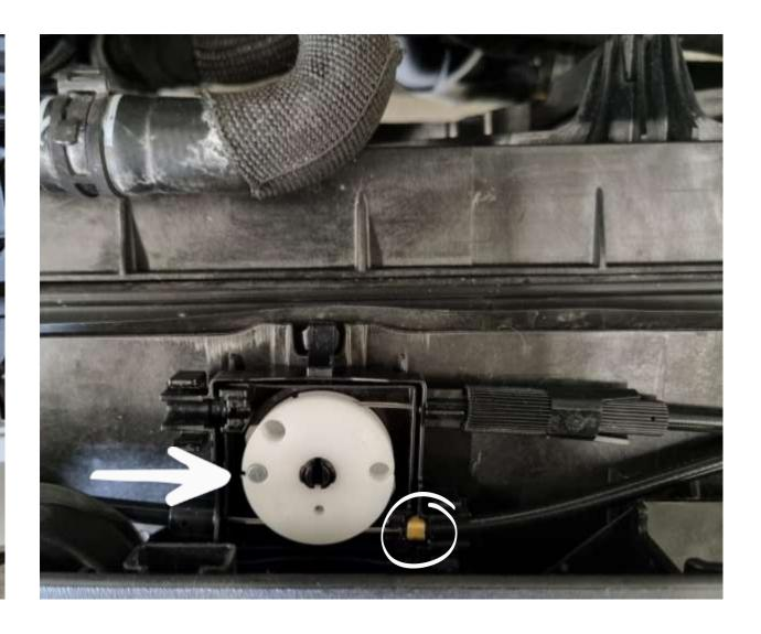
Disconnect 3x cable connectors and then loosen their cable fasterners with a small flat head screwdriver.
