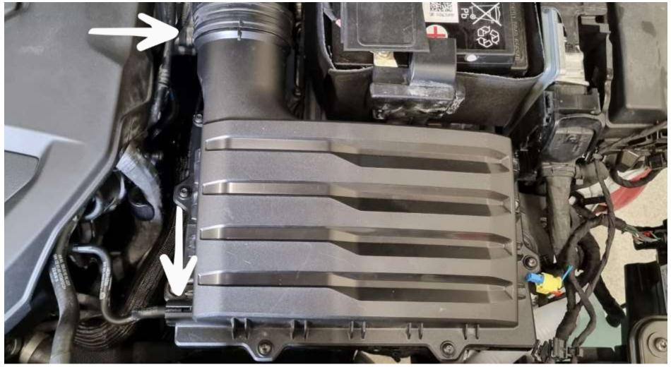
Remove 2x T25 screws to plastic air guide.
