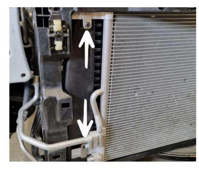
Use a small flat head screwdriver and loosen the plastic clips on the top of the AC condenser.
