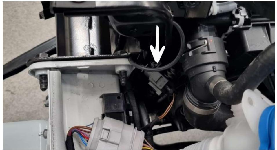
Remove 2x T30 and 2x 10mm hex screws and then remove the headlight from the car.
