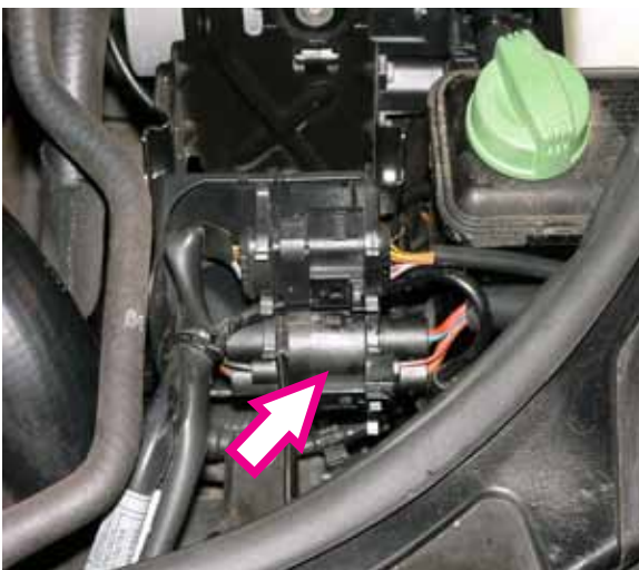
2. Separate the lower electric connector.
