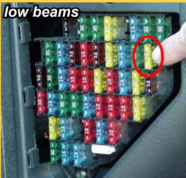
Remove fuse no. 15, Located at driver's side, at the left, inside the panel.
