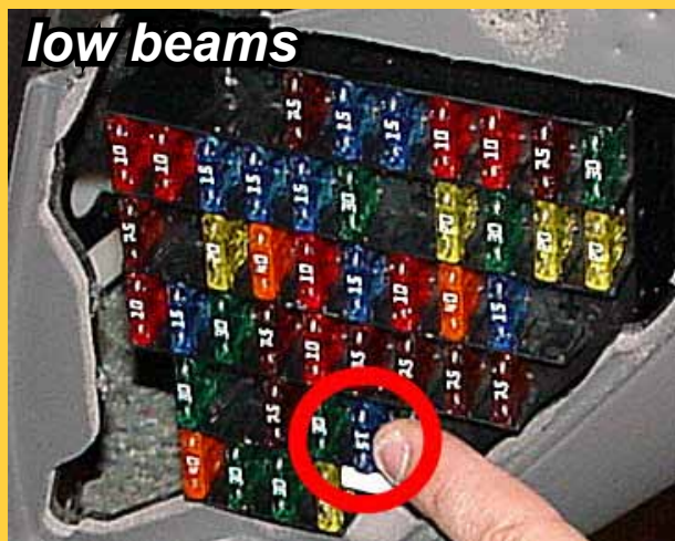
Remove fuse no. 35, located at driver's side, at the left, inside the panel.
