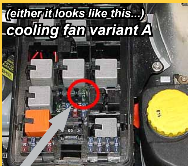
Remove fuse no. 35, located at driver's side, at the left, inside the panel.
