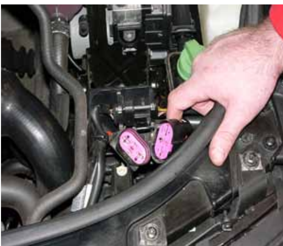
2. Separate the lower electric connector.
