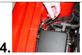
Remove the air box (3 attach points)
