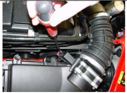
Remove the harness connector from the MAS.
