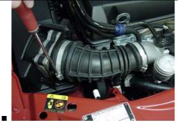
Remove the intake hose between the airpipe and the MAS (mass air sensor)
