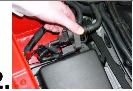
Remove the EVAP valve from the air box.
