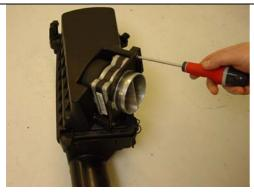
Remove the MAS from the air box, then remove the rubber packing from the MAS.
