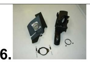
Assemble the MAS to the plate, notice the flow direction In picture 7. Use the original retaining plate with attached distances and screws.
