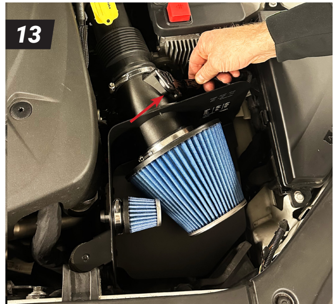
13. Connect the contact to the air mass meter tube.
