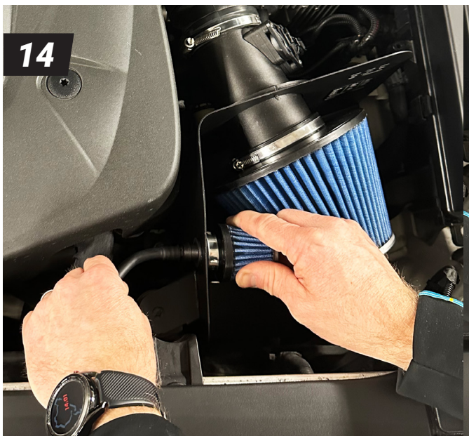
14. Install the hose in the connecting pipe. Rotate the connecting pipe to the correct position to fit. Install the clip. *Only applies to D5-engines.
