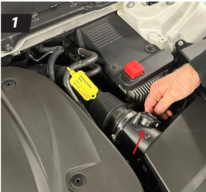
1. Disconnect the contact to the air mass meter tube.
