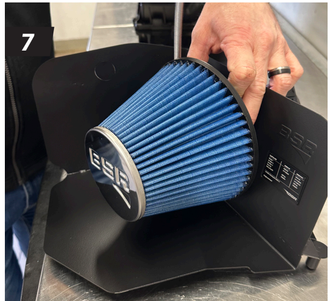
7. Install the air filter with the hose clamp. Do not tighten too hard.
