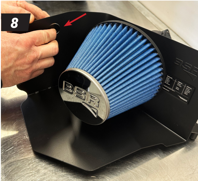
8. Remove the washer for the small air filter. *Only applies to D5-engines.
