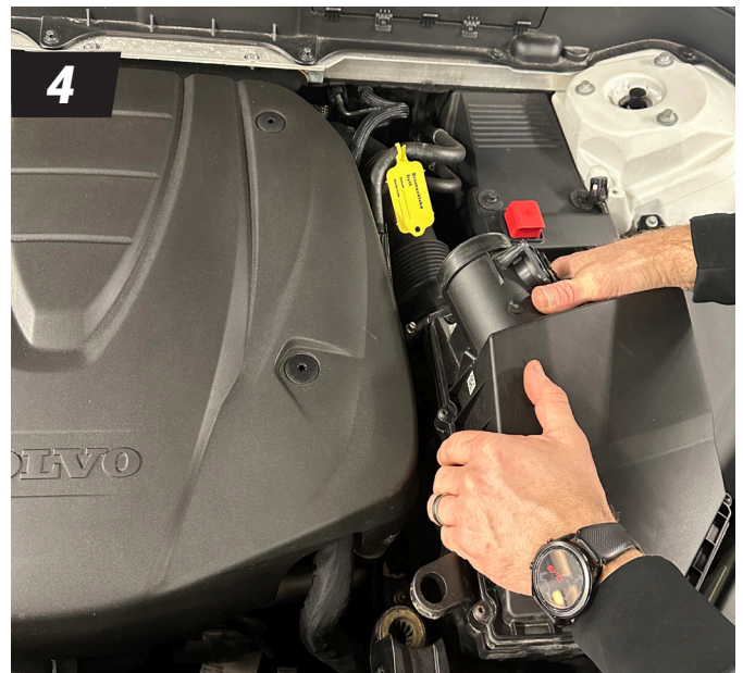
4. Remove the air hose. Grab the air box and pull it upwards.
