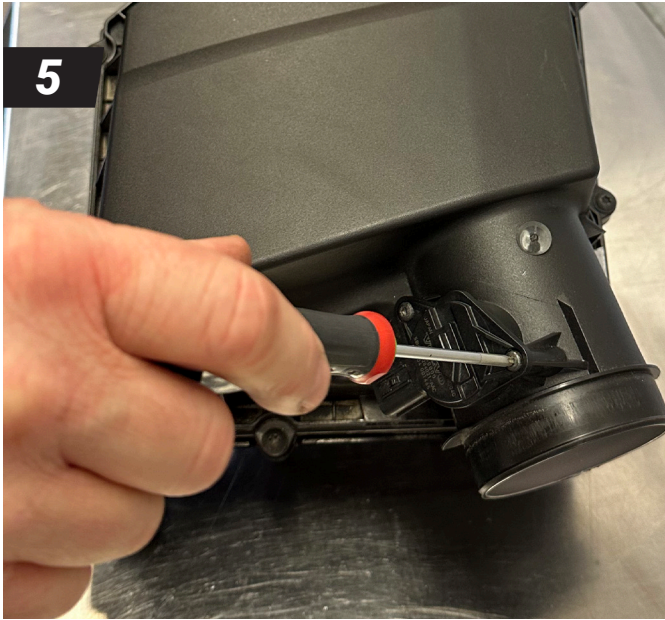
5. Transfer the air mass sensor to the new pipe with the existing screw (torx).
