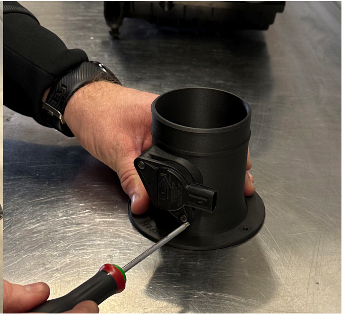
5. Transfer the air mass sensor to the new pipe with the existing screw (torx).
