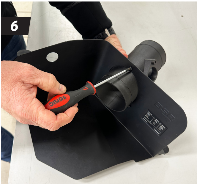
6. Install the pipes on the shield.
